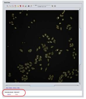
7 Capture an image and record the Intensity (Mean) value in a well where DRAQ5 is absent (-ve well).
